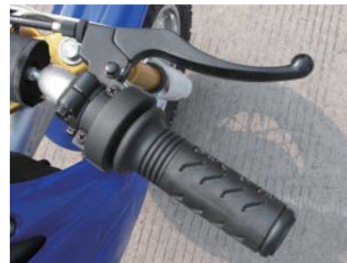
3、 The front wheel brake handle: front-wheel brake handle in the right hands. To handle its direction pinch Rafah as a front-wheel brake.
